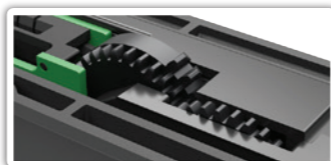
This picture shows the correct position of sector gear after rest.
